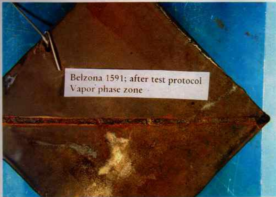
Figure 5. A close-up view of scribe : Test plate in the vapor phase.
