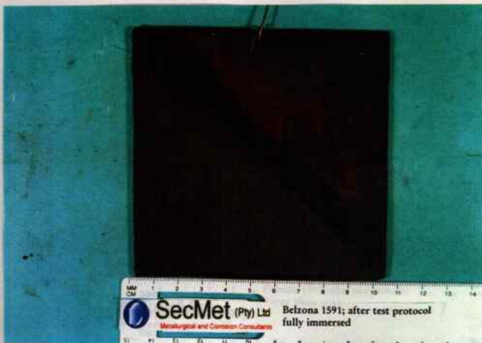
Figure 2. Belzona 1591 test panel after accelerated test protocol. : fully immersed
