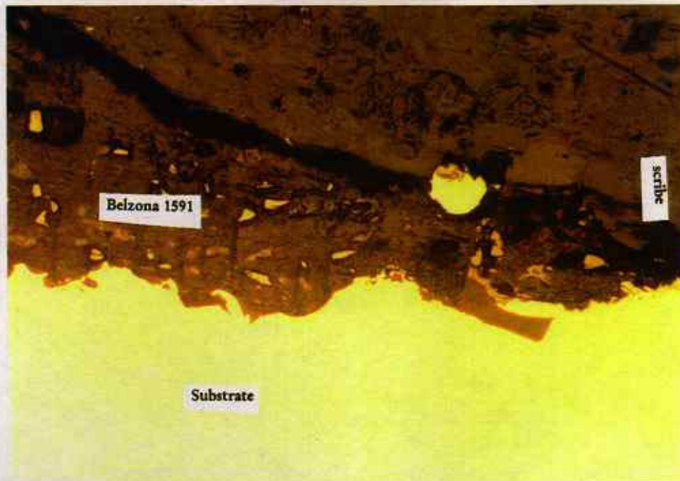
Figure 9. Micro-graph of coating system: vapor phase , Coating system still intact after test protocol (100X)
