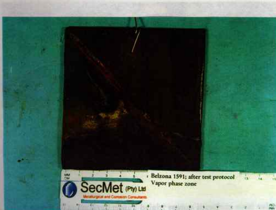
Figure 4. Belzona 1591 test panel after accelerated test protocol. : vapor phase
